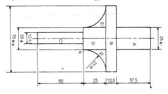
17. Estimate the time required to turn a 50 mm bar to the dimensions as shown in the figure below, with cutting speed 20 m/min and feed 0.7 mm/rev. Assume that all cuts are 2.5 mm deep. Neglect the facing time. All dimensions are in mm:
